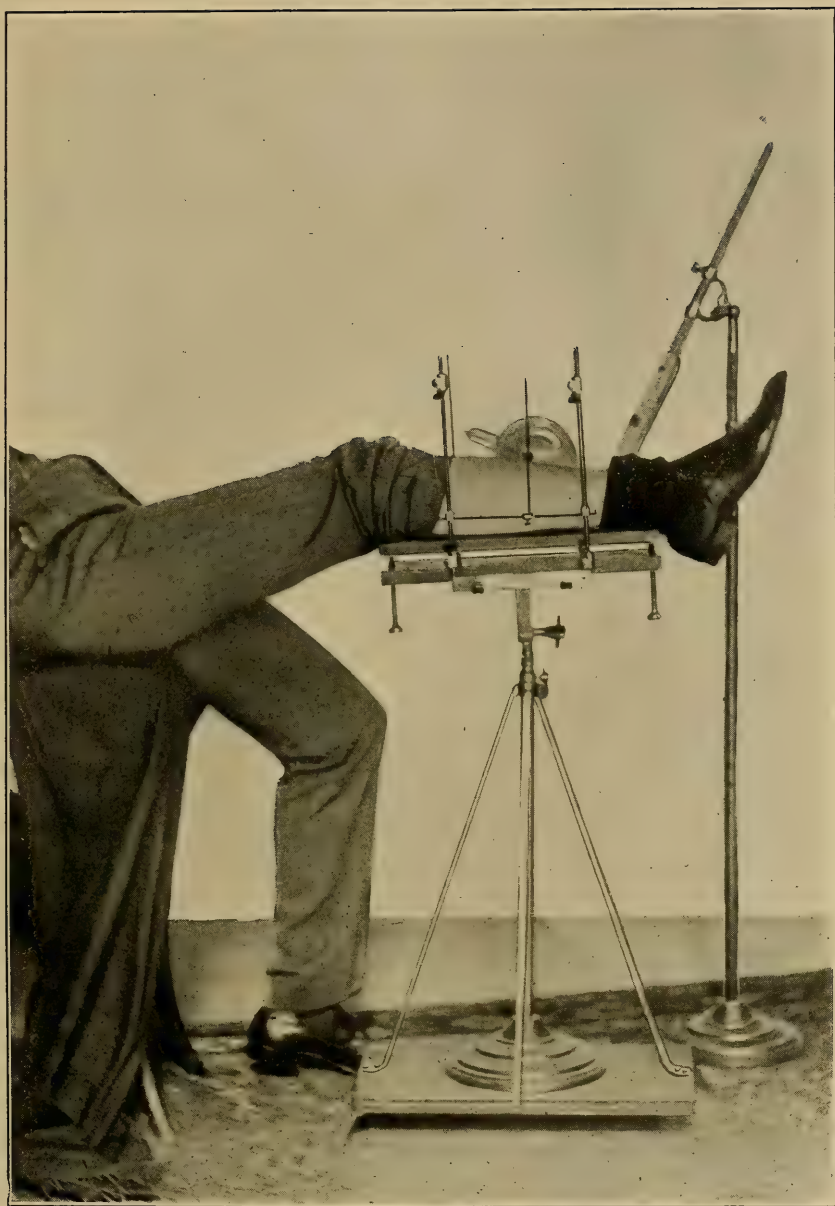
PLATE 61.—This instruction plate shows the Author's Examining Frame with its adjustable wooden floor used to level a part and support it during examination or localization. Turning the long spiral screws raises and lowers the upper shelf on which the part rests. Note the exact register of the two vertical guides in the axis of the rays. The central radiation coincides with the point where the horizontal and vertical guides intersect and the fracture, lesion; or bullet to be examined or located is seen without distortion when brought into this exact field. The plate teaches its technic at sight.
